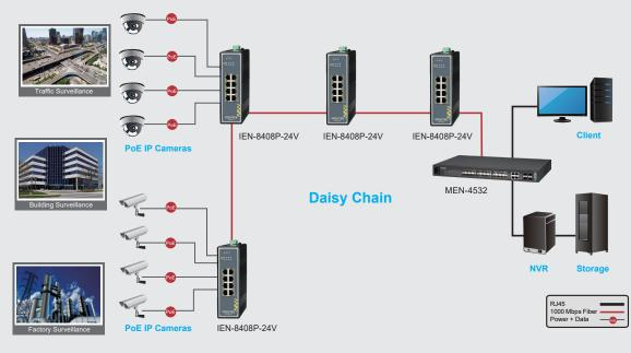
The IEN-8408P-24V is compatible with 10/100/1000Mbps through RJ45 transceivers to guarantee a strong, stable connection of Ethernet, Fast Ethernet or Gigabit Ethernet, providing flexible deployment options to satisfy industrial networking requirements.
