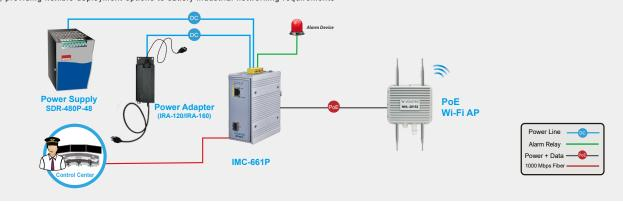
The IMC-661P combines high-power PoE+, robust performance for surveillance systems in harsh industrial environments. With its compact size, highly reliable and secure features ensure continuous operations in some special requirements for transportation, factory and outdoor places where high vibration degree, shock and wide range temperatures are present.
