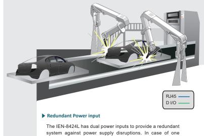
power source failure, the other acts as a backup to remain continuous network power for critical industrial applications.
