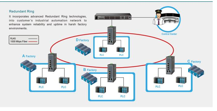
The INS-8624 is compatible with 10/100/1000Mbps through RJ45 transceivers to guarantee a strong & stable connection of Ethernet, Fast Ethernet or Gigabit Ethernet, providing flexible deployment options to satisfy industrial networking requirements
